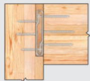
Housed in Primary Member (Column)
