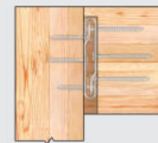
Housed in Secondary Member (Joist or Purlin)
