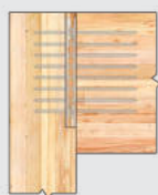
Housed in Primary Member (Column)
