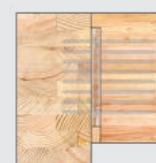
Housed in Secondary Member (Joist or Purlin)
