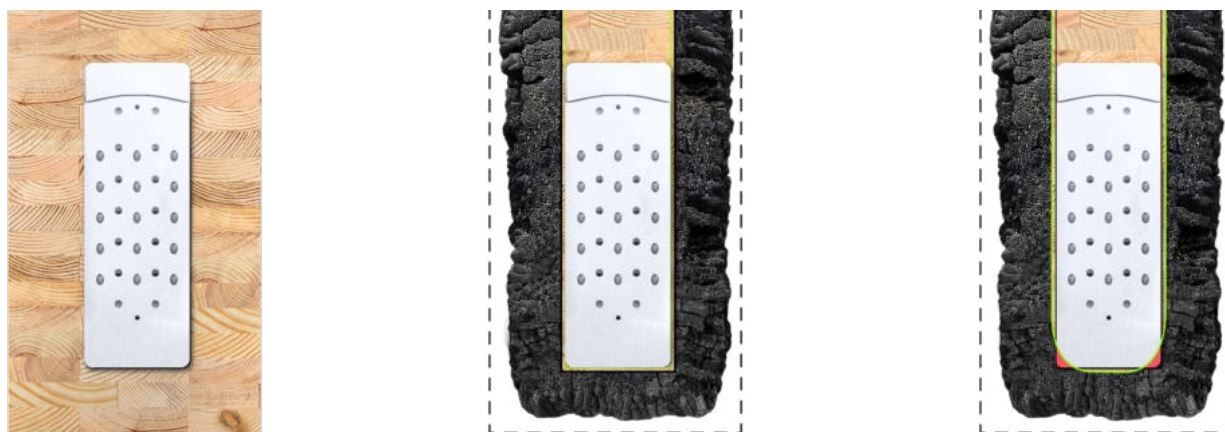
Figure A.5 - Corner Rounding Effects
