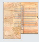
Housed in Secondary Member (Joist or Purlin)
