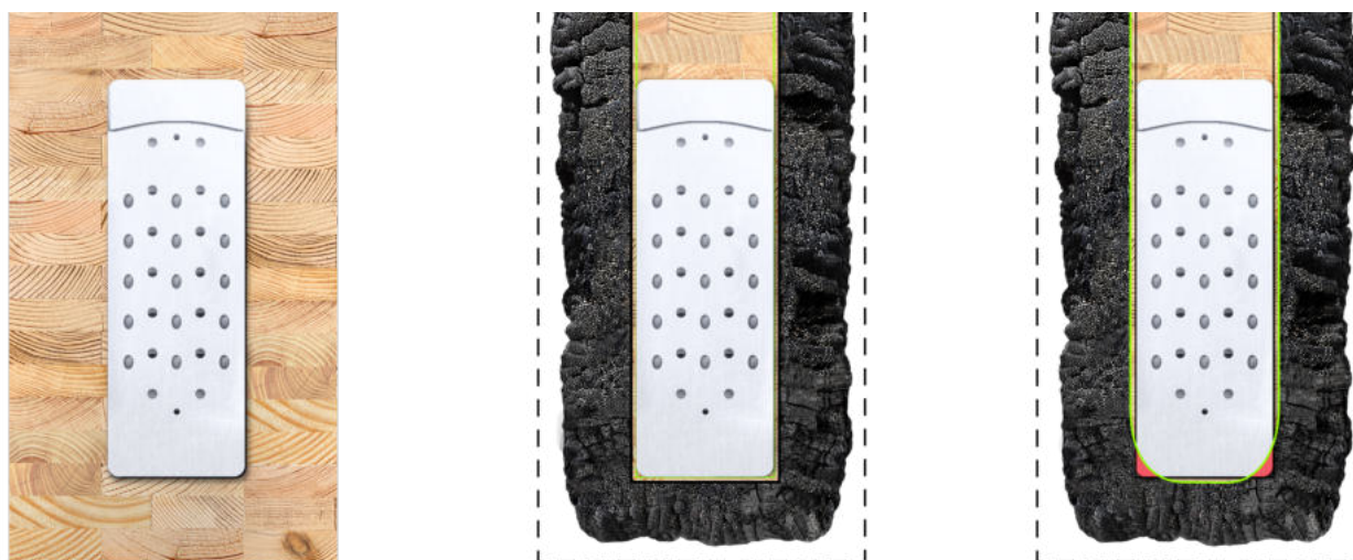
Figure A.2 - Corner Rounding Effects
