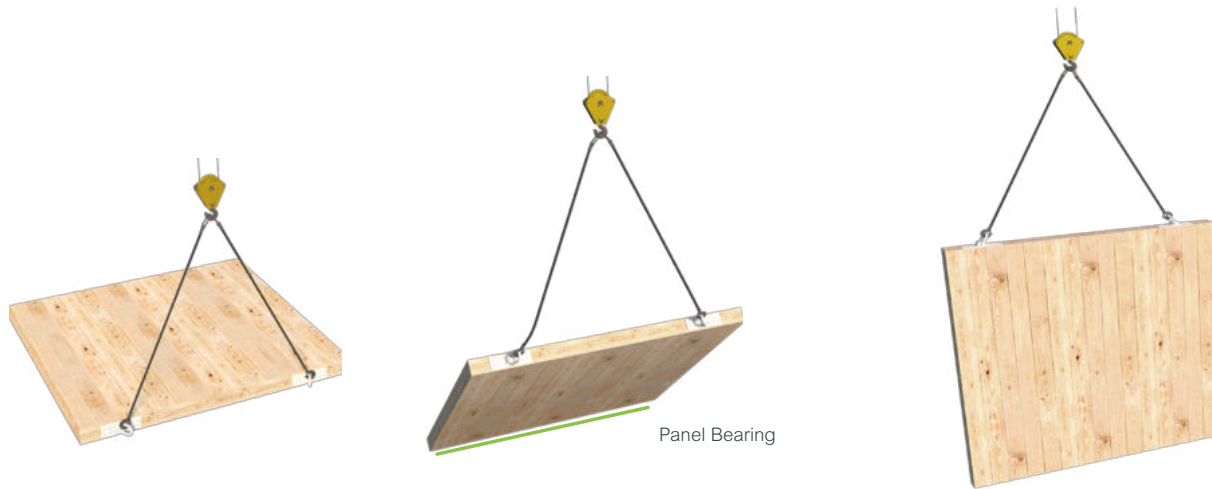
Tilting Up CLT Wall Panels with the Yoke XL
