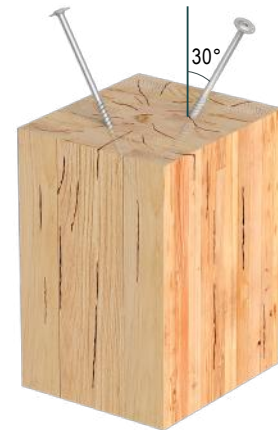
Dry, Checked Wood with Inclined Screws
