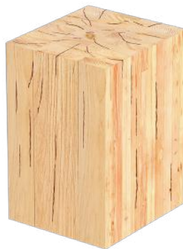
Dry, Checked Wood
