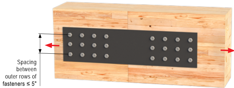
Maximum Spacing Between Outermost Fasteners
