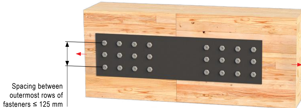
Maximum Spacing Between Outermost Rows of Fasteners
