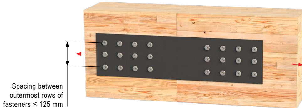
Maximum Spacing Between Outermost Rows of Fasteners
