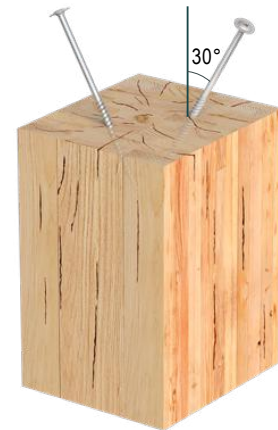
Dry, Checked Wood with Inclined Screws
