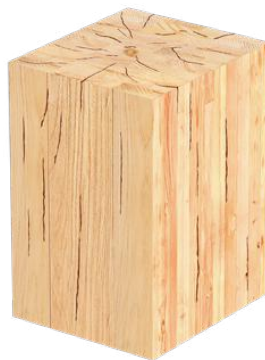
Dry, Checked Wood
