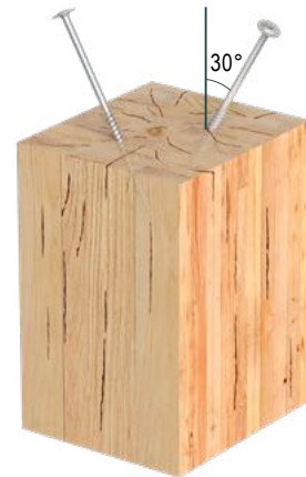
Dry, Checked Wood with Inclined Screws
