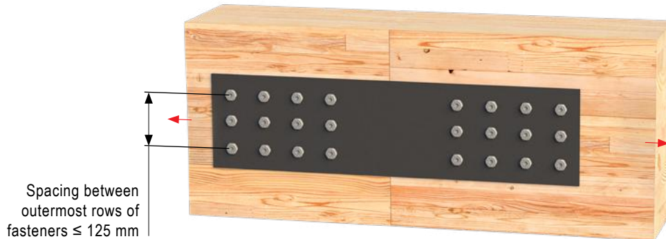
Maximum Spacing Between Outermost Rows of Fasteners
