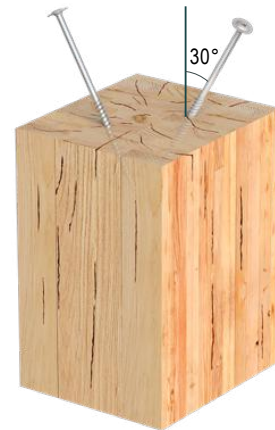
Dry, Checked Wood with Inclined Screws
