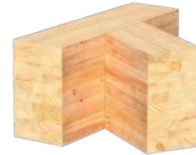
Skewed Configuration: Joist-to-Beam Connection
