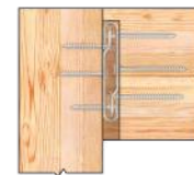
Housed in Secondary Member (Joist or Purlin)
