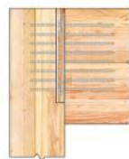
Housed in Primary Member (Column)
