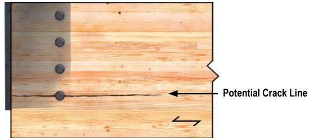
Figure C.3 - Lowest Dowel in Knife Plate Connection Does Not Support Bottom of Member
