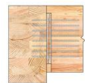
Housed in Secondary Member (Joist or Purlin)
