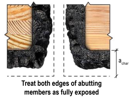
Figure A.3b - Char Contraction for Exposed Members
