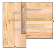
Housed in Primary Member (Column)
