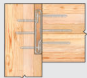
Housed in Primary Member (Column)
