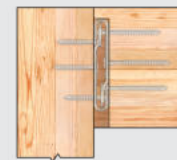
Housed in Secondary Member (Joist or Purlin)
