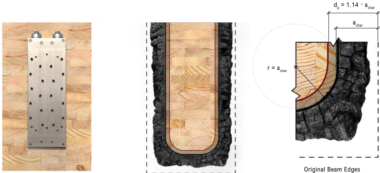
Figure A.5 - Corner Rounding Effects
