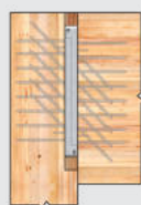
Housed in Primary Member (Column)
