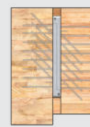
Housed in Secondary Member (Joist or Purlin)
