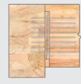
Housed in Secondary Member (Joist or Purlin)
