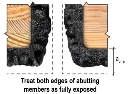
Figure A.3b - Char Contraction for Exposed Members Treat both edges of abutting members as fully exposed
