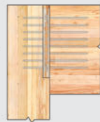
Housed in Primary Member (Column)
