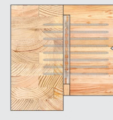
Housed in Secondary Member (Joist or Purlin)
