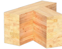
Skewed Configuration: Joist-to-Beam Connection
