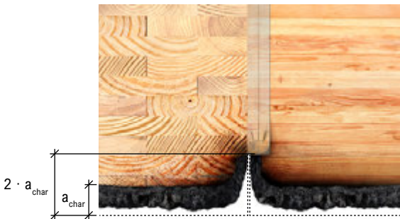
Figure A.3a - Char Contraction for Members \leq 1/8 in. Apart
