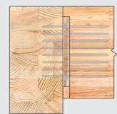
Housed in Secondary Member (Joist or Purlin)
