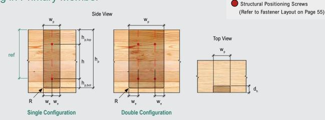
Table 2.21 - Routing Dimensions for RICON S VS Housed in Primary Member
