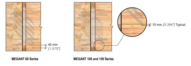
Figure A.6 - Distance Between Screw Tip and Connector for Megant
