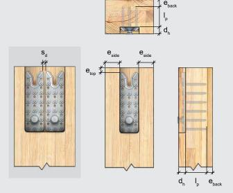
Table 2.9 - RICON S VS 60 Geometry Requirements for Primary Member (Column)
