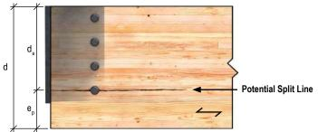
Figure C.3 - Lowest Dowel in Knife Plate Connection
