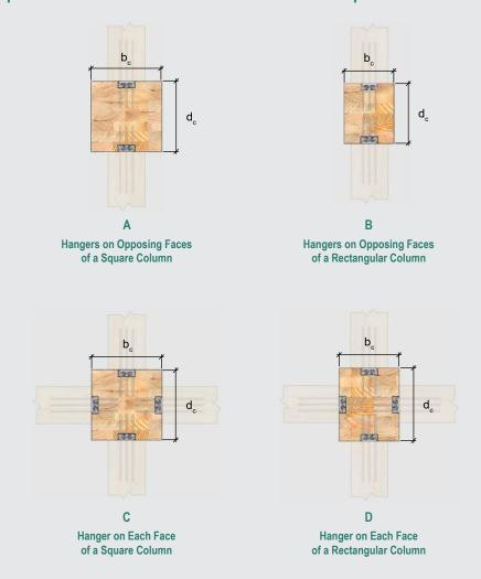
Table 2.18 - Minimum Column Sizes for Multiple RICON S VS Connectors
