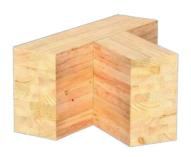
Skewed Configuration: Joist-to-Beam Connection
