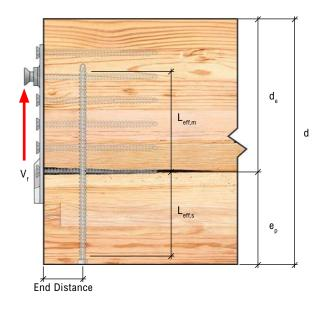
Figure C.10 - Reinforcement Placement in Beam-End
