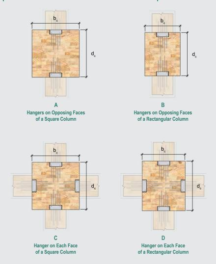
Table 4.11 - Minimum Column Sizes for Multiple APEX Connectors
