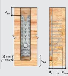
Table 2.16 - RICON S VS XL 390 x 80 Geometry Requirements for Primary Member (Beam/Girder)
