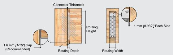
**Routing Depth:** The routing depth is the depth of the housing,  $d_h$ , noted in the Geometry Requirements and Housing Dimensions sections. This depth takes into account the thickness of the connector and the gap between members (recommended 1.6 mm [1/16 in.] herein—larger gaps will reduce  $d_h$  accordingly).
