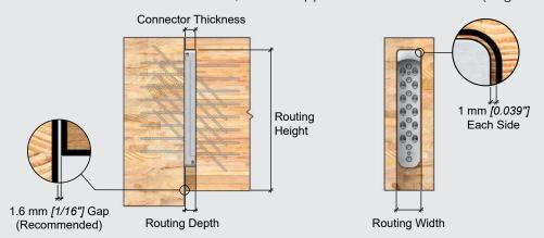
**Routing Depth:** The routing depth is the depth of the housing,  $d_h$ , noted in the Geometry Requirements and Routing Details sections This depth takes into account the thickness of the connector and the gap between members (recommended 1.6 mm [ 1/16 in. ] herein—larger gaps will reduce  $d_h$  accordingly).
