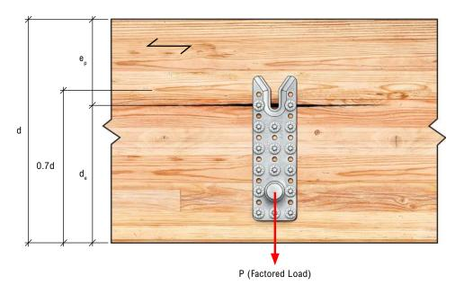
Figure C.1 - Splitting at Low Connection on Primary Member's Side
