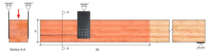
Figure C.7 - Splitting of Beam Supported Near its End
