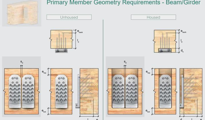
Table 4.9 - APEX 150 Geometry Requirements for Primary Member (Beam/Girder)
