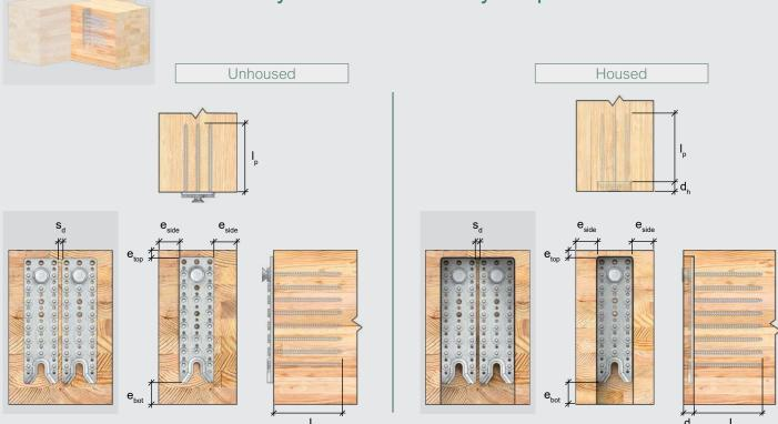
Table 2.11 - RICON S VS 80 Geometry Requirements for Secondary Member
