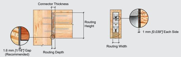
**Routing Depth:** The routing depth is the depth of the housing,  $d_h$ , noted in the Geometry Requirements and Routing Details sections. This depth takes into account the thickness of the connector and the gap between members (recommended 1.6 mm [ 1/16 in. ] herein—larger gaps will reduce  $d_h$  accordingly).
