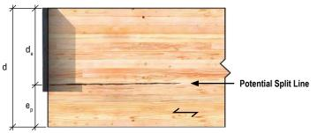
Figure C.2 - Concealed Bearing Plate Does Not Support Bottom of Member
