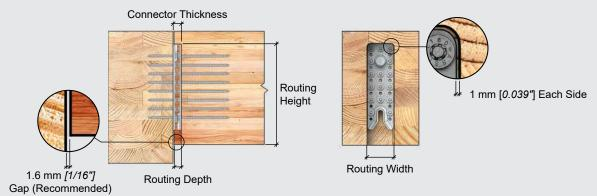
**Routing Depth:** The routing depth is the depth of the housing,  $d_h$ , noted in the Geometry Requirements and Routing Details sections This depth takes into account the thickness of the connector and the gap between members (recommended 1.6 mm [ 1/16 in. ] herein—larger gaps will reduce  $d_h$  accordingly).
