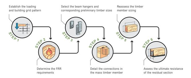
Figure A.1 - Proposed Member Sizing Design Flow
