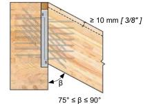
Sloped Configuration: Rafter-to-Ridge Beam Connection (Side View)
