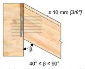
Sloped Configuration: Rafter-to-Ridge Beam Connection (Side View)
