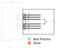
Figure C.12 - Reinforcing Screw Placement for Avoiding Screw Collisions
