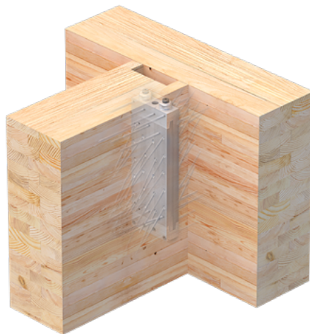
Figure 2. Example of a Concealed Fire-Rated Connection with a MEGANT Connector
