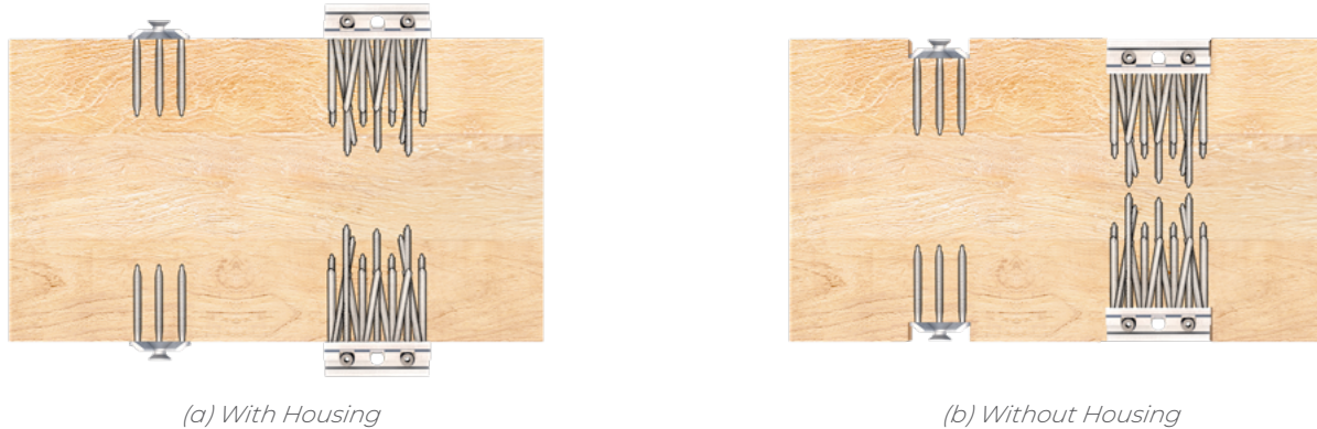
Figure 7. Top View of a Typical Girder Beam
