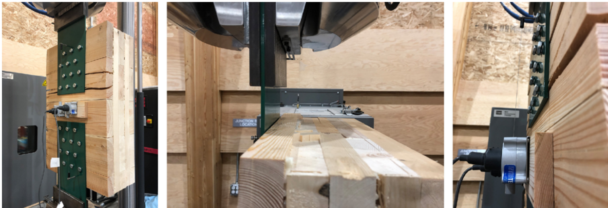
Figure 2. Rolling and Plug Shear and Splitting Failure Observed in a CLT Panel Subjected to Splitting Force Component
