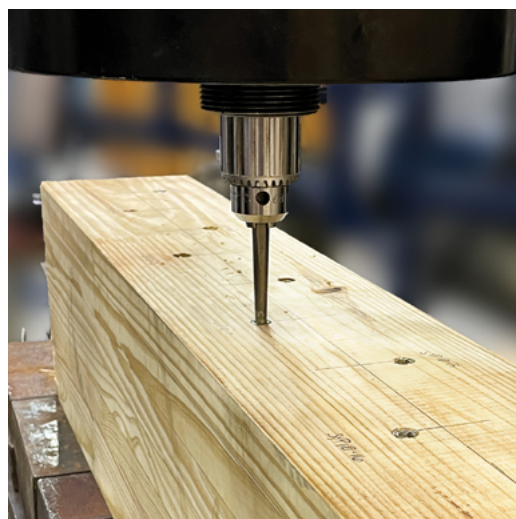
Figure 1. Tapered Punch Direct-Load Application to the Head of the Screw in Glulam
