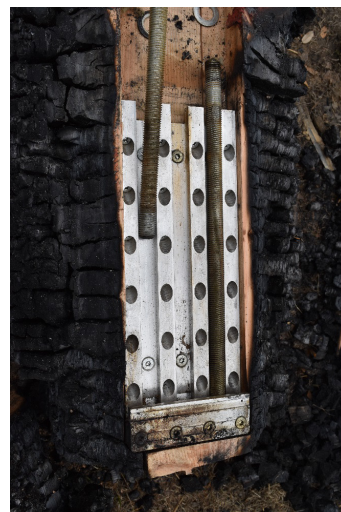
RICON S VS and MEGANT Connectors After Fire Testing
