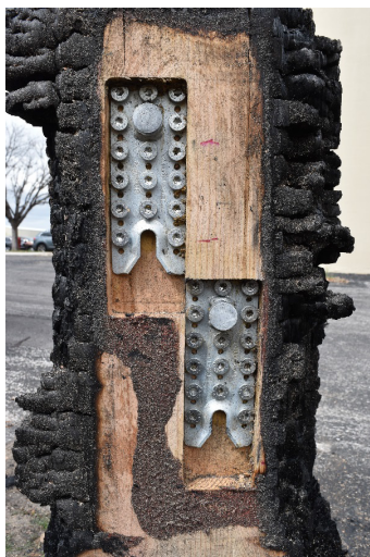
RICON S VS and MEGANT Connectors After Fire Testing
