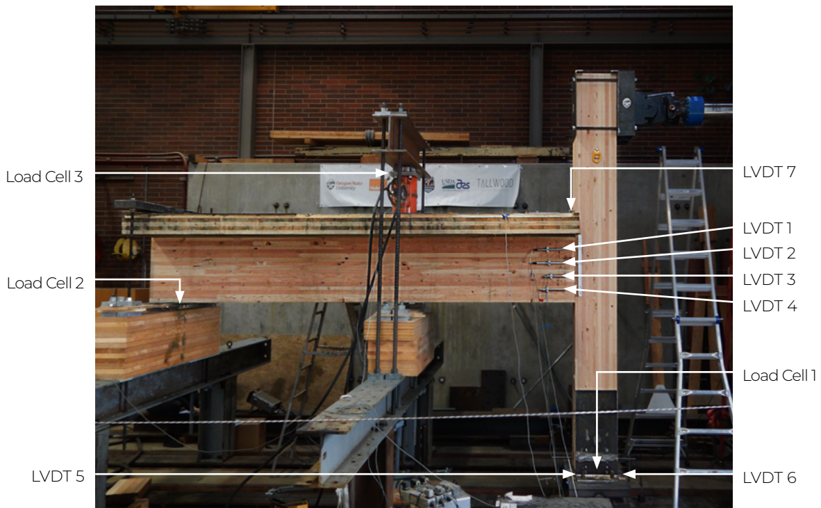
Figure 2. Specimen Sensor Layout
