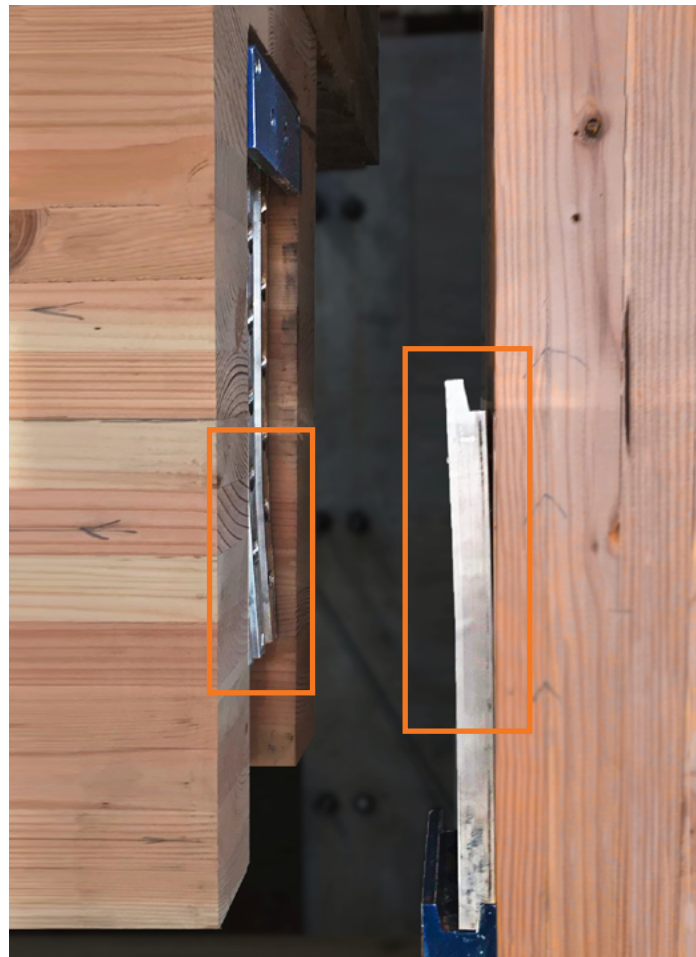
Figure 12. Typical Connector Plate Bending Failure Under Cyclic Test
