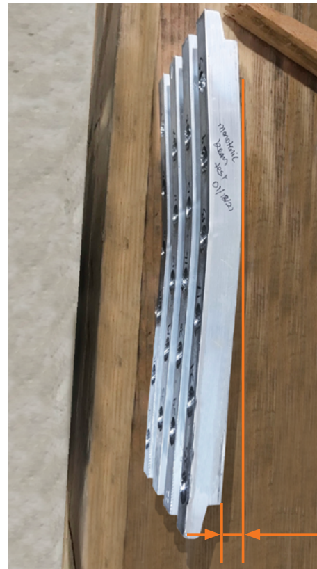
(b) Typical Connector Plate Bending Failure Under Monotonic Test
