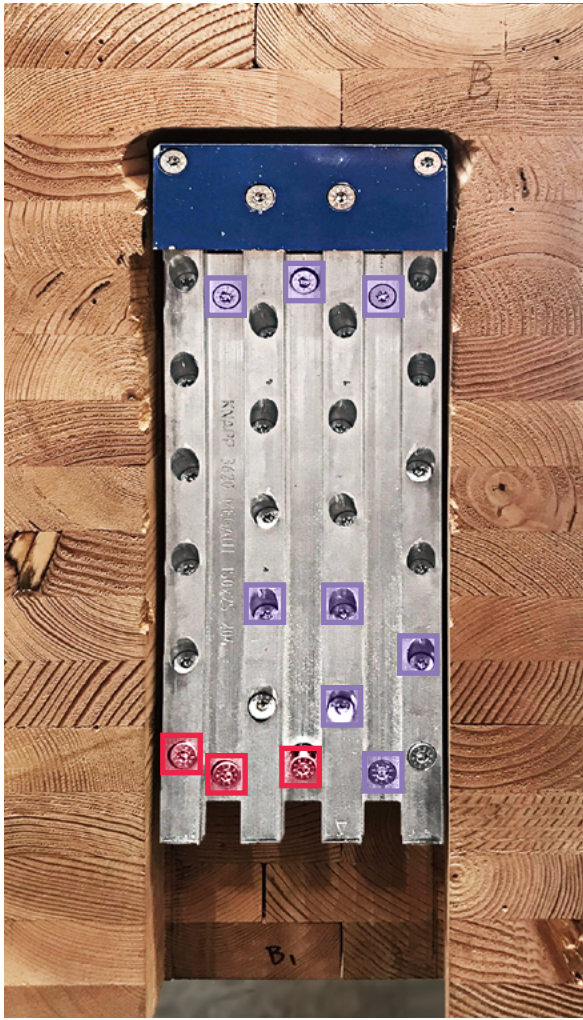
Tensile Failure Withdrawal Failure
