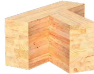
Joist to Beam Connection
