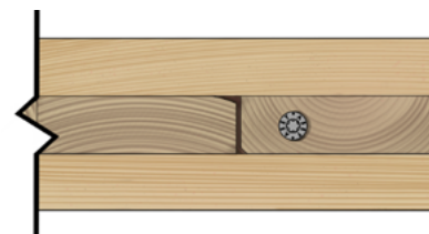
Screw Installed in the Narrow Edge
