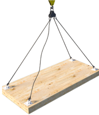
Example of uneven load sharing
