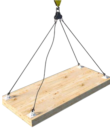
Example of uneven load sharing
