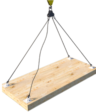
Example of uneven load sharing
