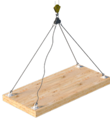
Example of Uneven Load Sharing
