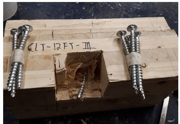
Figure 3. Cutaway of the test specimen to reveal the deformed shape of the ASSY® screws and localized embedment failure (left: Kombi; right: VG CSK) after testing to failure. [Pictures provided by University of Alberta research team].
