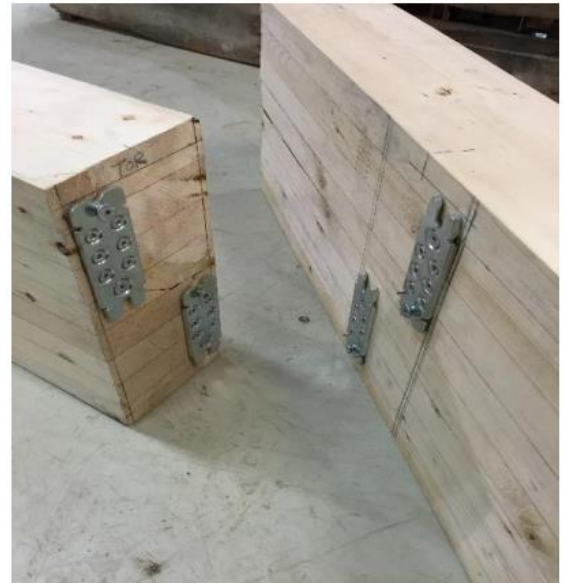
Double Ricon Joint Configuration (Matthew Ficara©)
