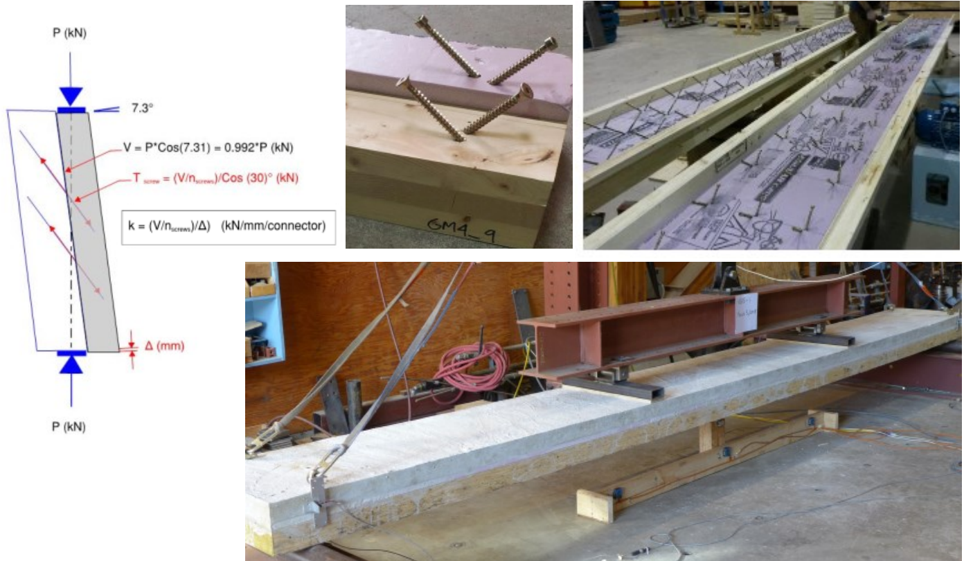
Figure 5: Test Setup of the Shear Test: schematic (left) and picture (right) as per [3]
