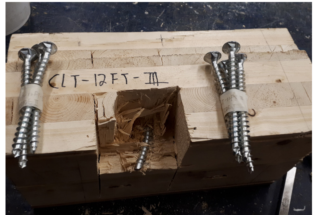
Figure 3. Cutaway of the test specimen to reveal the deformed shape of the ASSY® screws and localized embedment failure (left: Kombi; right: VG CSK) after testing to failure. [Pictures provided by University of Alberta research team].
