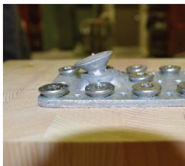
FIGURE 17, Yielding of collar bolt.
