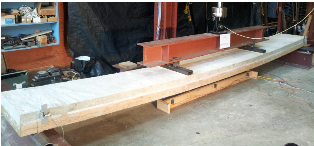
Fig.2– TCC Floor system under testing at the Univ. of British Columbia [5]
