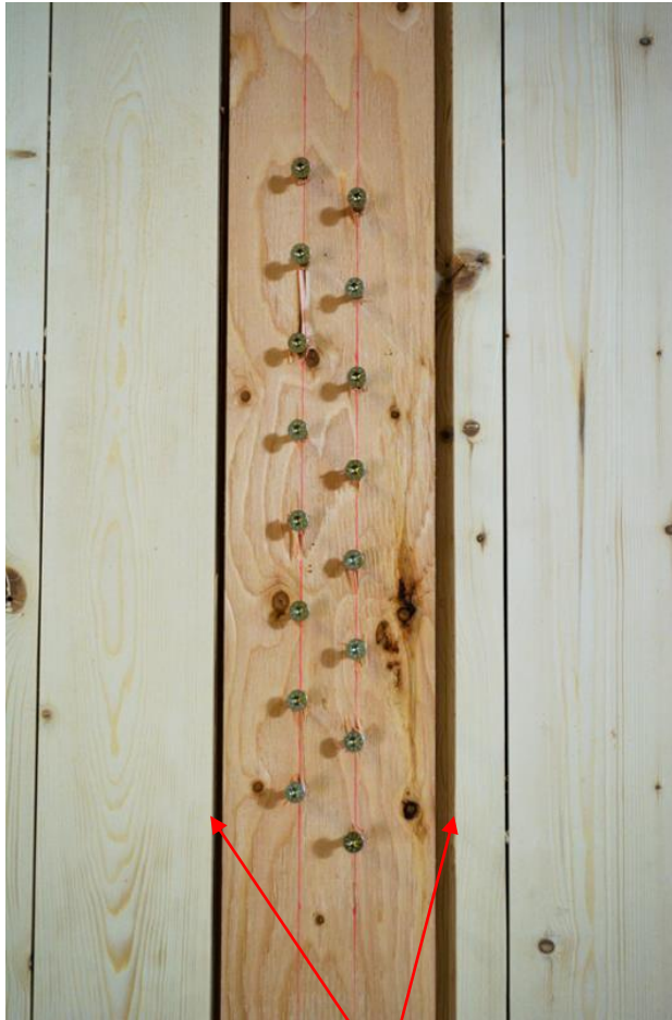
Separation of members in ultimate state
