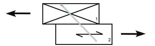
Looking at the screw capacity alone, the only effect would be that in member 1, the withdrawal capacity would be higher, since the angle to the grain ( $\alpha$ ) is 90 degrees. For member 2, the angle to the grain ( $\alpha$ ) would be whatever angle the screw is installed relative to the shear plane.
