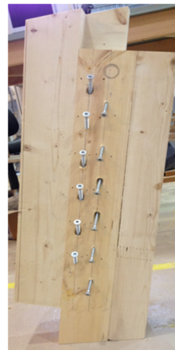
Half Lap Joint Specimen
