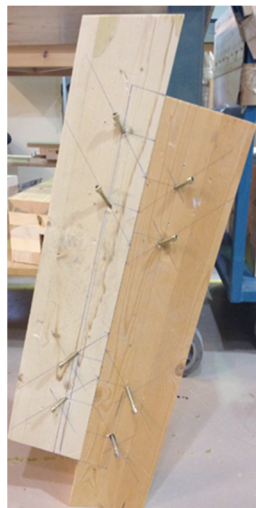
Butt Joint Specimen
