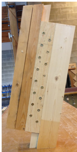
Surface Spline Joint Specimen
