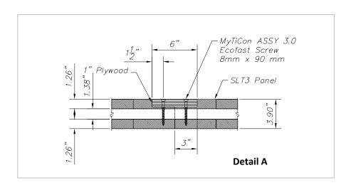
Screw Diameter, D = Major Diameter = 8.0 mm (0.315 in.) **NOTE:** Minimum end distances, edge distances Shank Diameter = 5.8 mm (0.228 in.)Minor Diameter = 5.3 mm (0.209 in.)Screw Length, L = 90 mm (3.54 in.)
