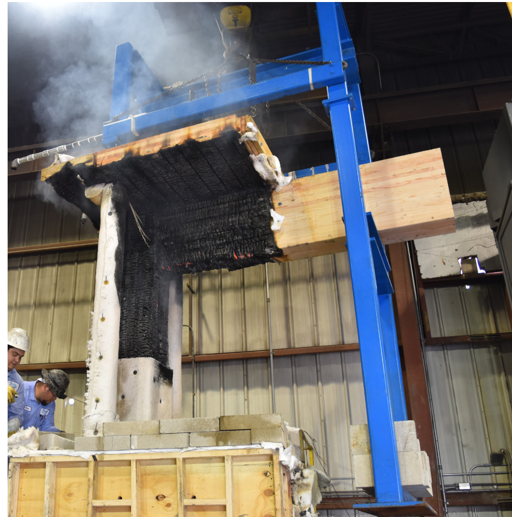
Fire Rating with Char Layer
