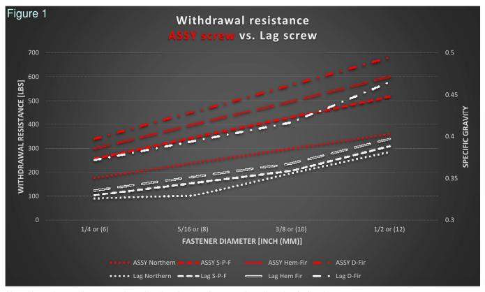
Note: Above chart applies to screw-in angles of 90° between fastener axis and wood grain direction
