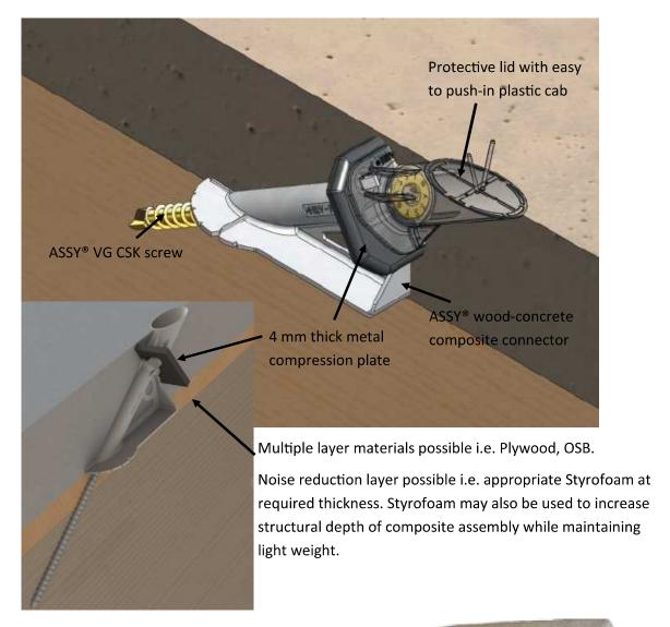
Bearing of screw head on metal compression plate. Metal plate transfers compression stress into concrete.
