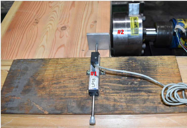
Figure 3: Displacement recording (#1) at interface of beam and column and constant design shear load application actuator (#2)
