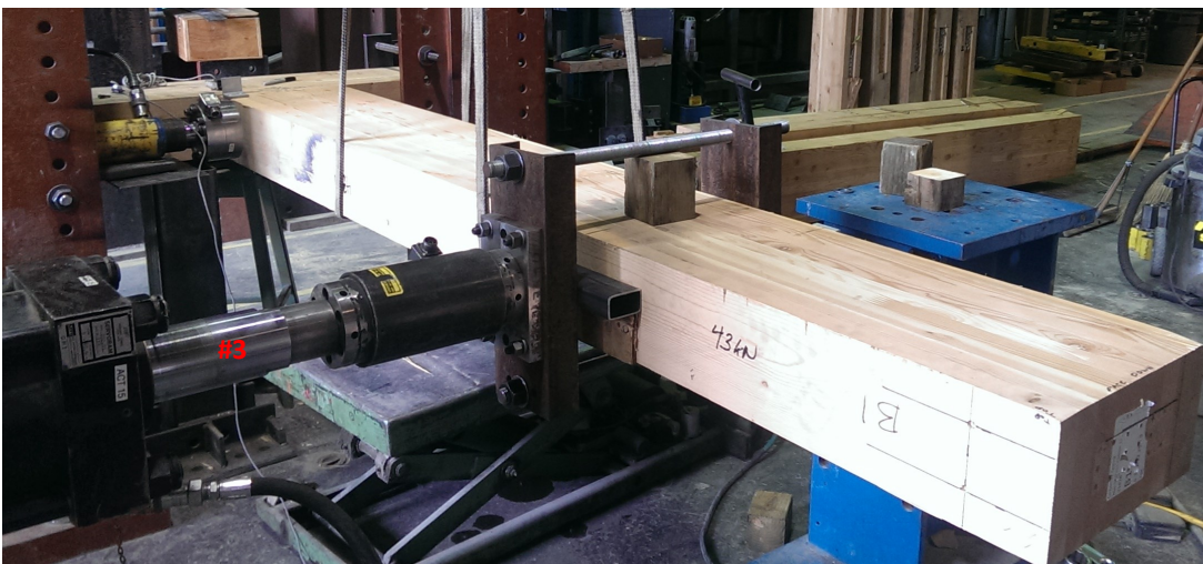
Figure 5: Displacement application actuator (#3) at 65 1/4" away from interface of beam and post
