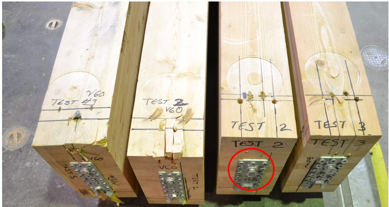
Figure 9: Example of collar bolt failure at maximum drift and load in beam member Ricon S VS 200x60 in 2 out of three tests. Figure 10: Example of collar bolt yielding at maximum drift and load in beam member RICON S VS 200x80 in 3 out of three tests
