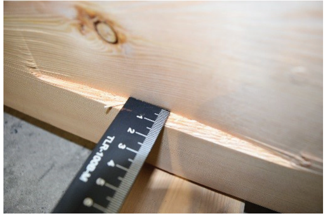
FIGURE 12, Bottom of dummy test beam after dummy test without compression reinforcement.
