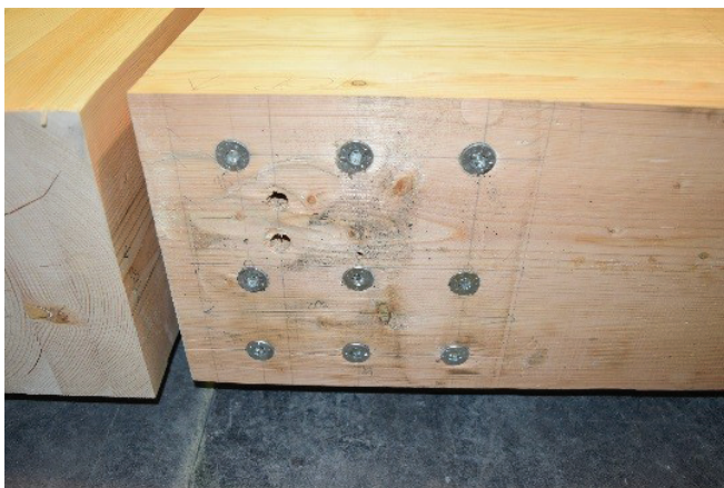
FIGURE 9, Top of beam after test with compression reinforcement.
