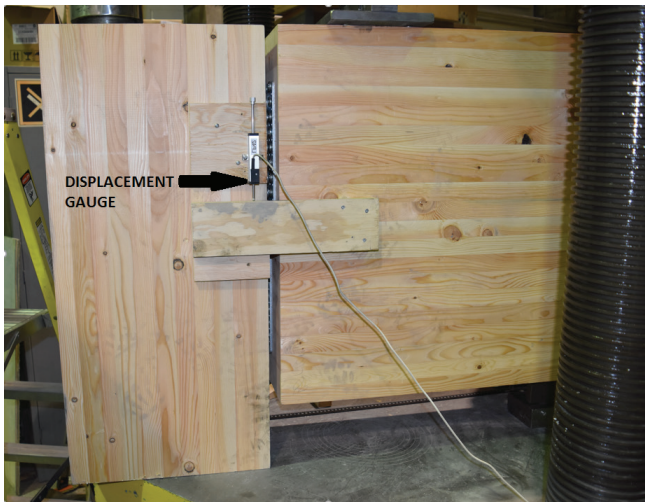
FIGURE 13, Test setup (column left, beam right) showing one of two symmetrically placed displacement gauges.
