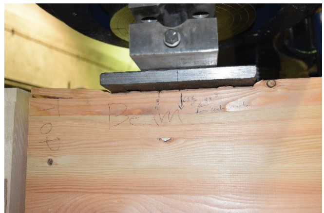
FIGURE 10, Top of dummy test beam after test without compression reinforcement.
