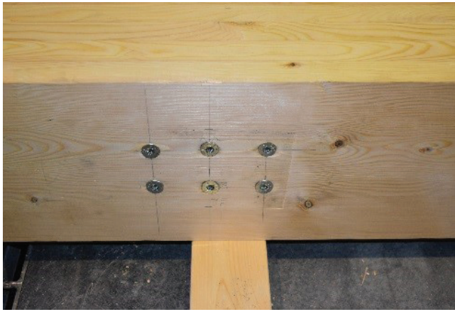
FIGURE 11, Bottom of beam after test with compression reinforcement.
