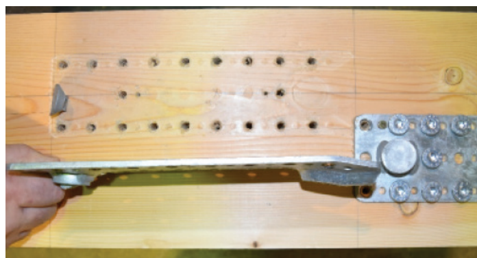
FIGURE 19, Condition of wood after testing. No wood embedment failure evident.
