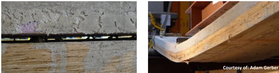
Fig. 18. Series 2 panel failure due to screw withdrawal (left) and timber tensile failure (right) - Brittle [5]
