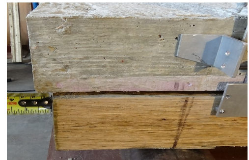
Fig.7 – Slip at ends of composite sections after reaching ultimate capacity
