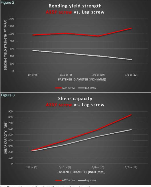
Note: Shear capacity compared for main and side member loaded parallel to grain
